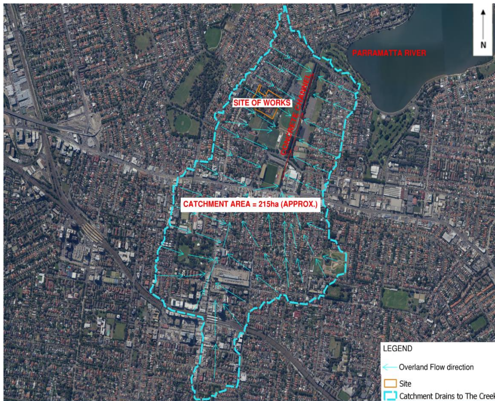
Figure 4 – Upstream Catchment of Concrete Channel
